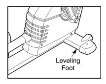
ing use, turn one or both of the leveling feet under the front stabilizers until the rocking motion is eliminated.
